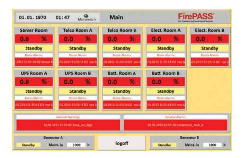
The control unit may be enabled to communicate with a building management system installed on site by Modbus TCPIP protocol via standard Ethernet cable. Alternatively, the system can be upgraded to be monitored and
